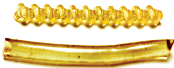
Figure 3. Example of melt fracture (top strand) exhibited by KSPS and NaSPS when the extrusion process was accelerated. The bottom strand is an example of the strands used for the extensional tests.
